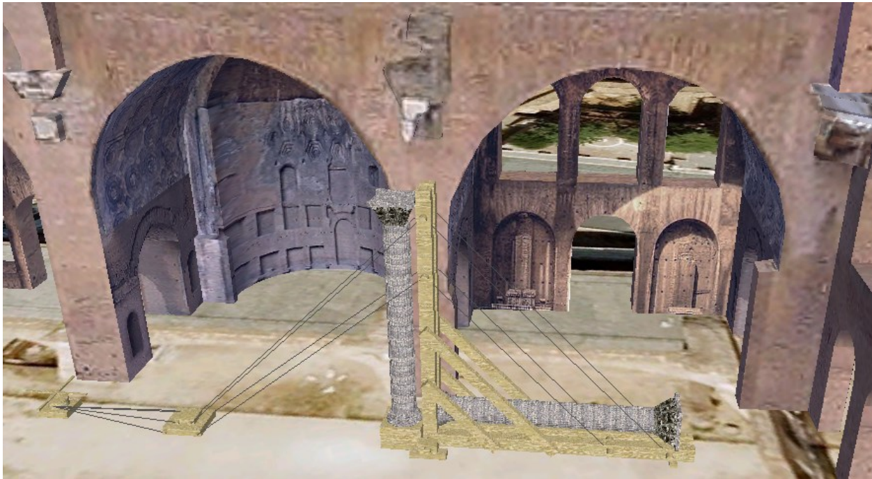
Fig. 4: Superimposition of 3D model of lifting machine by the author after the descriptions of Vitruvius and the drawing by J.-P. Adam, inserted into a GoogleEarth framework with 3D buildings enabled (including Basilica of Maxentius for scale).
