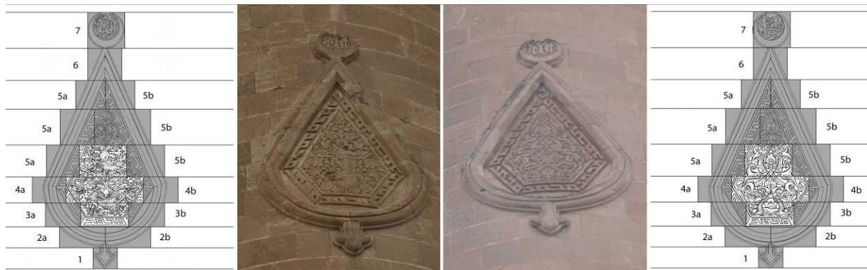
Fig. 14: Mapping of joints and ashlar shape for the drop shape medallions.
