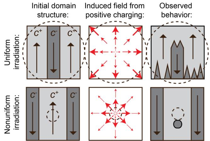
FIG. 4. Schematic showing electric fields due to positive sample charging, alongside observed domain behavior. The dashed circles represent the area of electron irradiation. The arrows in the left and right panels represent ferroelectric polarization, and the arrows in the middle panel represent the induced electric field.
