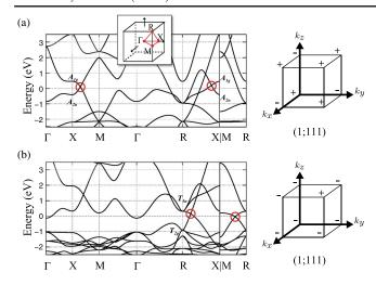
FIG. 2 (color online). Electronic structures and  $\mathbb{Z}_2$  indices of (a)  $Cu_3NZn$  and (b)  $Cu_3NPd$ . Bands are drawn along the high-symmetry lines of the Brillouin zone (inset). The Dirac points are indicated by red circles. Parity eigenvalues are illustrated at the eight parity-invariant points in the first octant of the BZ.
