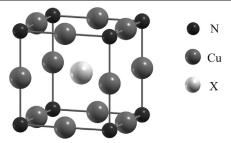
FIG. 1. Crystal structure of  $Cu_3NX$ . X represents a transition metal atom intercalated at the body center of the cubic unit cell of  $Cu_3N$  in an anti-ReO<sub>3</sub> structure.
