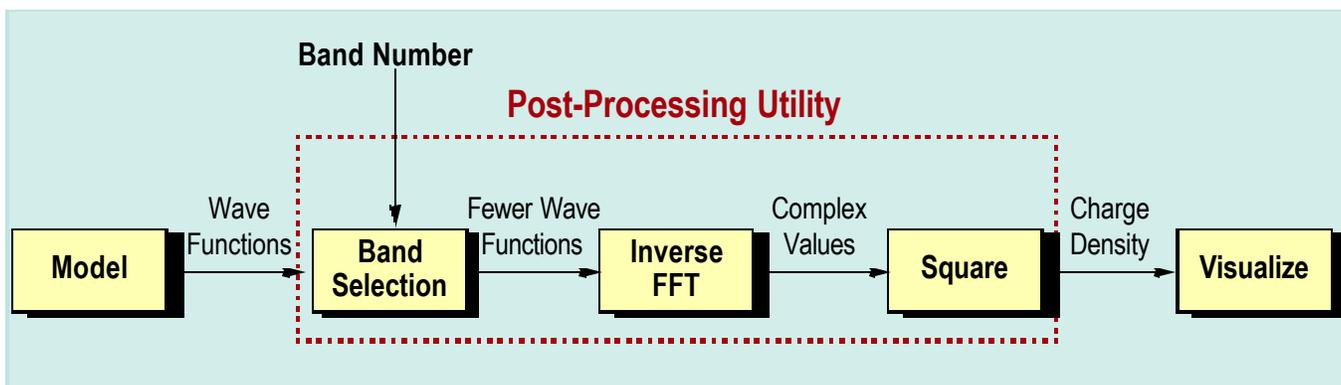
**Figure 1. Step-by-step diagram of the Post-Processing Utility.**
