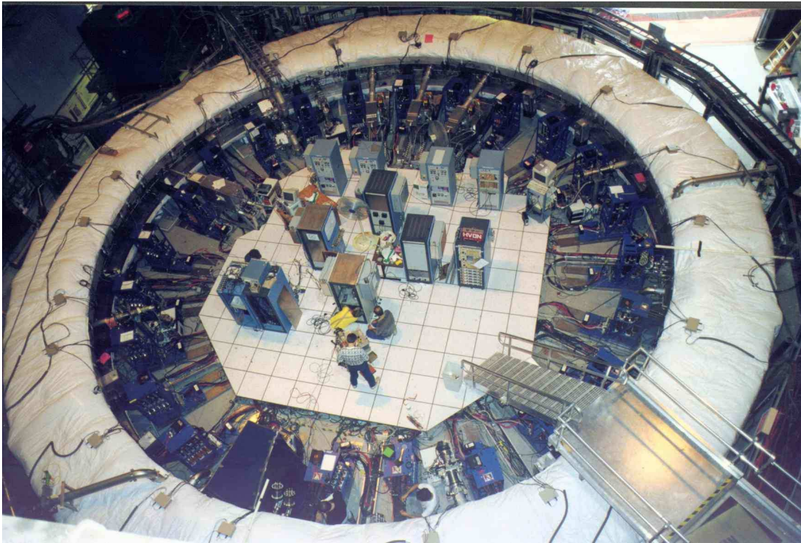
Figure 3.4: Photograph of the muon (g-2) storage ring with the thermal insulator.
