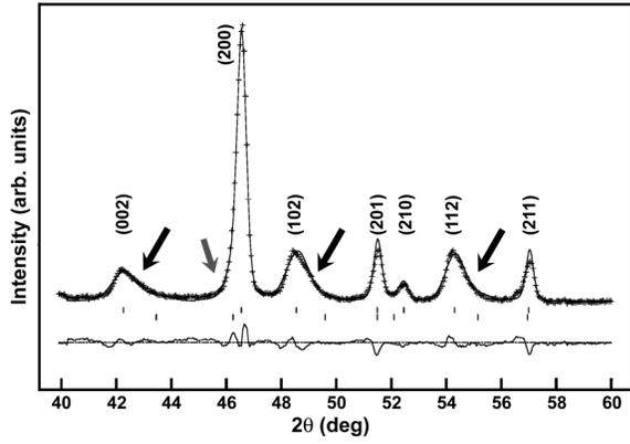
FIG. 1. Experimental and refined neutron diffraction data plotted in the  $40^\circ$ – $60^\circ$   $2\theta$  range for the  $x = 0.35$  composition. Crosses indicate experimental data, two-phase fit shown by solid line and fit difference is marked at bottom. Black arrows point to asymmetric broadening of  $l$ -containing peaks, while the gray arrow highlights the more subtle  $h, k$  peak broadening.
