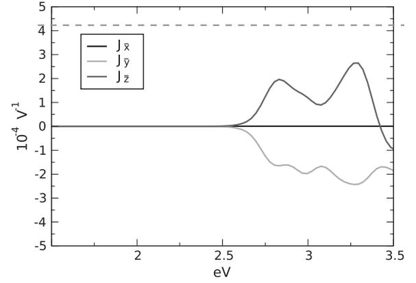
FIG. 7. The calculated current densities per light intensity in the lab frame of the BFO film, with the experimental value from Ref. [3] marked by the dashed red line. The current in the  $\bar{x}$  direction, parallel to the domain walls, vanishes, while much of the remaining current is directed toward the bottom of the sample.
