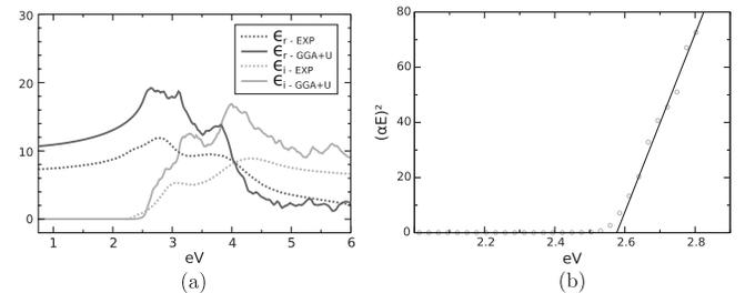
FIG. 2. In (a), the calculated components of the permittivity,  $\epsilon$ , are compared to experiment. In (b), the calculated band gap is shown to be 2.58 eV, 0.16 eV less than the experimentally determined value of 2.74 eV [22].
