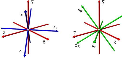
FIG. 6 (color online). The relationship between the principal axes of the material coordinates and the lab coordinates ( $\bar{x}$ ,  $\bar{y}$ ,  $\bar{z}$ ) in Fig. 4. The  $z_R$  and  $z_L$  axes are parallel to the polarization in their respective domains; the  $x_R$  and  $x_L$  are in the  $\bar{x}$   $\bar{z}$  plane; and  $y_R$  and  $y_L$  complete the orthogonal bases.
