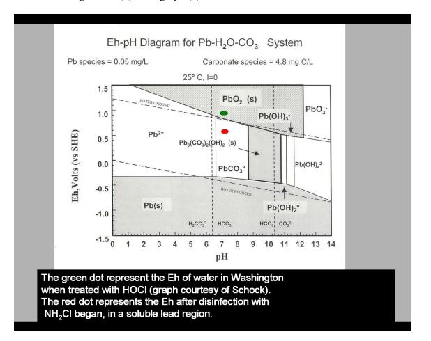
To remove the lead (make it insoluble, as in the grey regions of the graph above), the pH would have to be increased by adding a base, or the oxidative potential would have to be increased.
